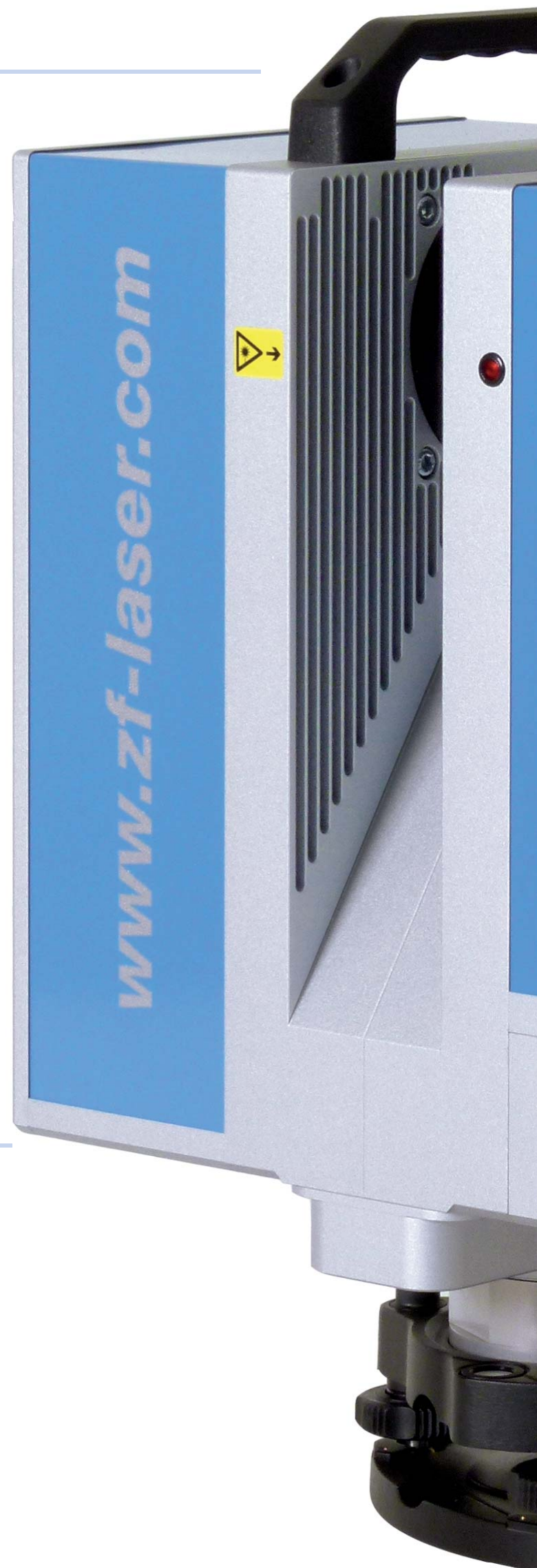
Rotating mirror for 310° vertical scanning
